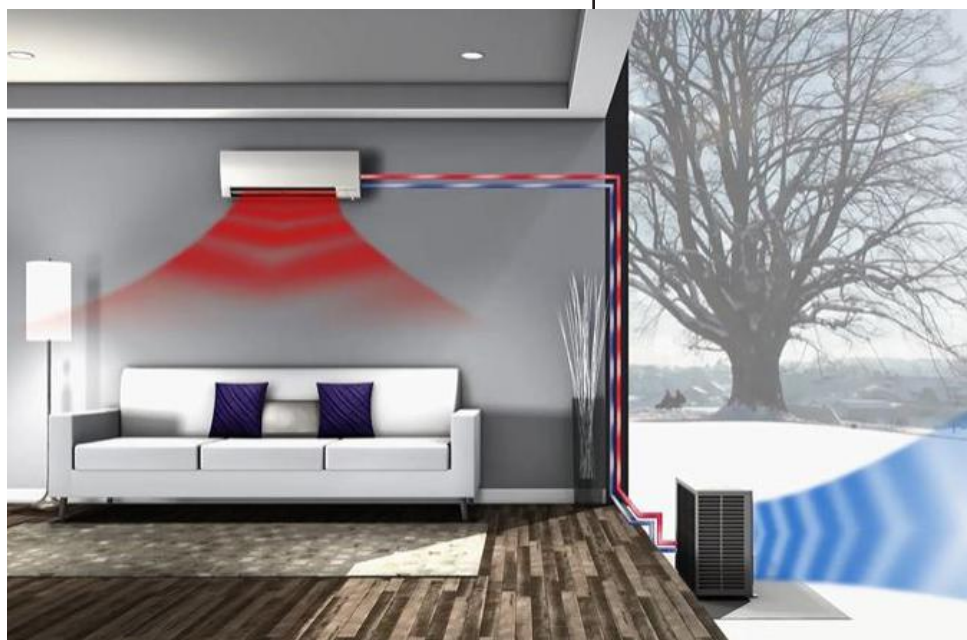
Diagram of the heat transfer between the outdoor unit and indoor unit during heating operation
